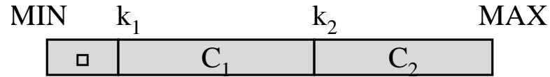
Figure 4.5 : Tuple authenticated dictionary showing 2 keys and 3 tuples. Tuple ([k_j, k_{j+1}), c_j) is represented as a rectangle from k_j to k_{j+1} containing c_j .
